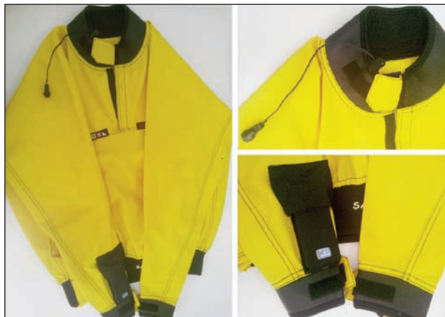
Fig. 7. Electronically equipped sailing garment (left: whole garment, right top: collar and the heart rate sensor clip, right bottom: the slave module inside water-roof pocket)
